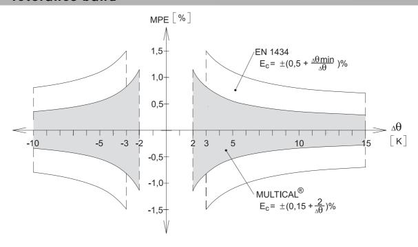
The above diagram shows MULTICAL®'s tolerance band, compared with tolerance requirements in EN 1434,
